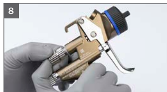
8 Install material flow control screw
