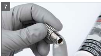
7 Grease thread of material flow control screw
