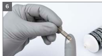
6 Grease and insert paint needle spring
