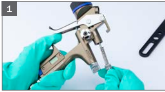
1 First remove paint needle.
